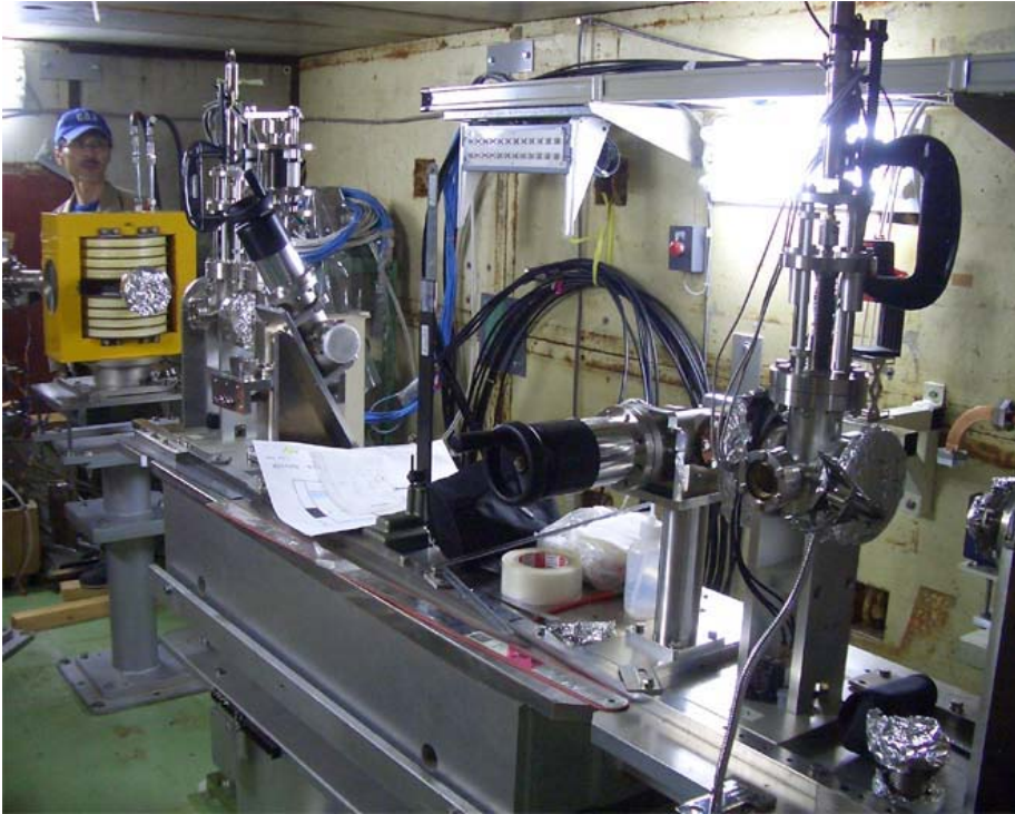
Girder for structure and beam-line components
